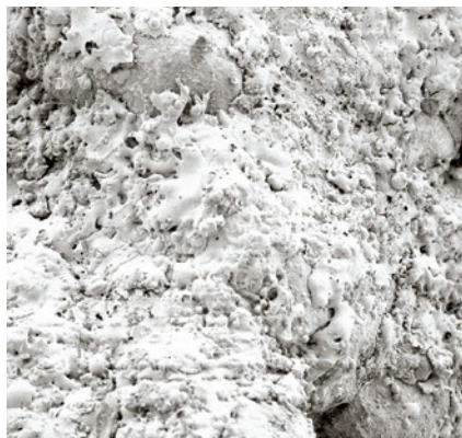
SEM images of an HA-sprayed surface
